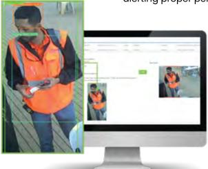
action can be taken. This is achieved though the utilisation of real-time electronic RFID tags. This unique identification feature can identify workers who do or do not comply with PPE standards, increasing the implementation of site safety monitoring around exclusion zones and machinery safe distancing.
